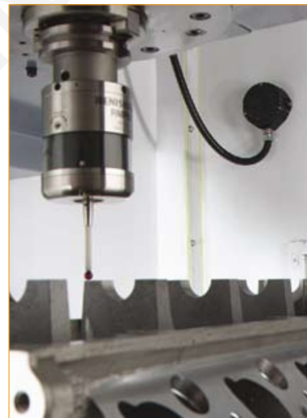
RMP60 probe inspecting a component, with RMI receiver / interface in the background
