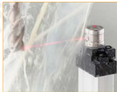
NC4 checking a tool for breakage with coolant running
